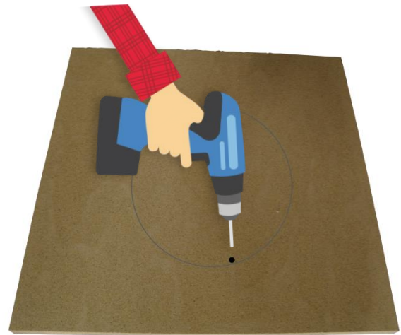
2. Pre-drill a groove for the jigsaw with a cordless screwdriver / drill.
