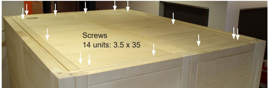
Fig. 18: Attaching the roof element
