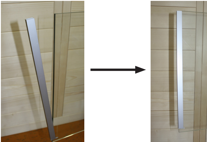
Fig. 10: Attach the U-profiles to the glass plates
