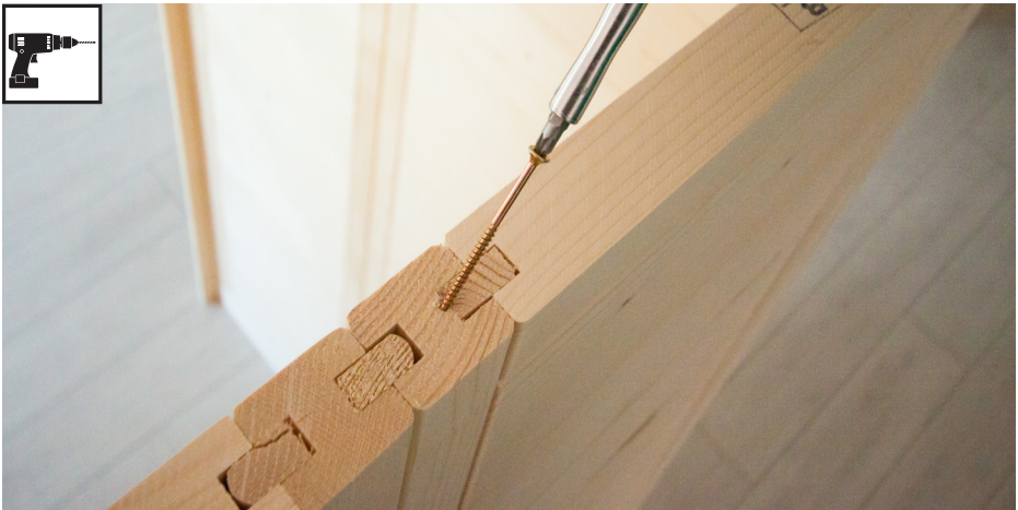
3 mm drill bit, 8 screws 4 x 70 mm
